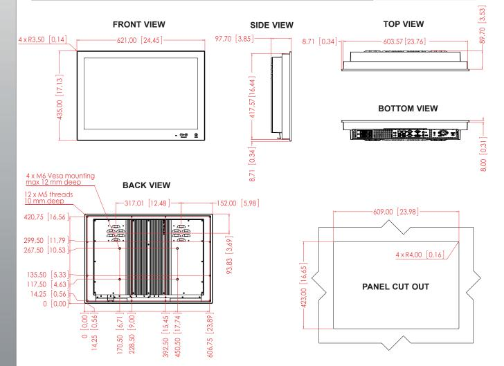
Dimensions might be shown with or without decimals and indicated as mm [inches]. Tolerance on drawings is +/- 1mm. For accurate measurements, check relevant DWG file.
